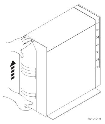
Figure 1. Remove System Unit Back Cover
